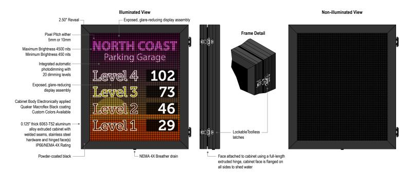
Outdoor/indoor blank-out signs with an IP66/NEMA 4X cabinet, narrow angle LEDs and contrasting black face. The sign message is formed by visible LEDs that illuminate when activated and blank-out when deactivated
